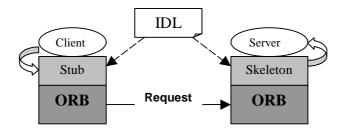
Figure 5. Stub and skeleton files
